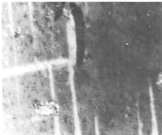
Figure 7 Crack at the end of a stopped twin, formed at -95^\circ\text{C} . The crack is 30 \mu\text{m} long, with an opening of \sim 3 \mu\text{m} , \times 850 .
