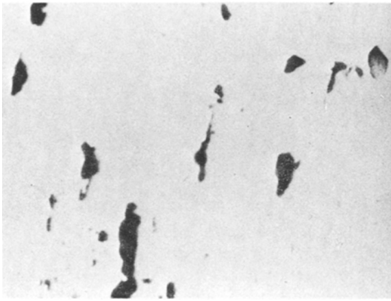
Figure 8 Transgranular voids formed in a slow tensile test at 500° C and a strain rate of 10^{-3} \text{ sec}^{-1} . The voids are strongly elongated, as in Fig. 6, \times 700 .
